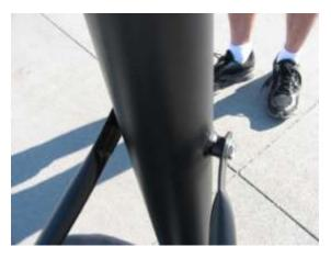
9. Next, attach (2) POLE BRACES to the threaded attachments on the LOWER POST and to the BASE TANK attachment holes as shown. Each POLE BRACE attaches to the LOWER POST using (1) 5/16" x 5/8" hex bolt and (1) 5/16" washer. The POLE BRACES attach to the BASE TANK using (1) 5/16" x ¾" hex bolt, (2) flatwasher and (1) 5/16" locknut. (place a flatwasher on top and bottom side of BASE TANK when attaching POLE BRACE)
