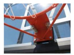
21. Using (2) 5/16" x 1 ½" hex bolts, (4) flat washer and (2) 5/16" lock nut, attach FLEX GOAL (BOTTOM HOLES) to BACKBOARD and BACKBOARD MOUNT.
