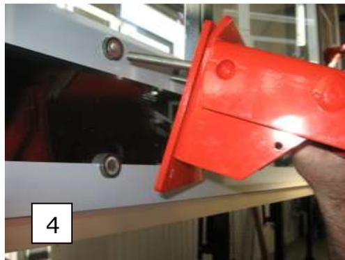
5. Insert bottom two carriage head bolts into place and finger tighten using flatwashers, lockwashers and hex nuts. (Add flatwashers, lockwashers and hex nuts if threaded studs are located at lower attachment points)
