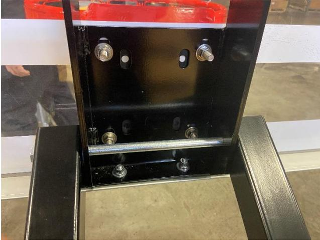
15. IF YOU PURCHASED A TEMPERED GLASS BACKBOARD, check once again to make sure all (4) grommets are in place in the backboard rim mounting holes. When you are satisfied with rim hole/H-Frame alignment, attach rim following the instructions provided in the rim box. Then tighten the 5/16" hardware at both the top and bottom of the backboard frame.
