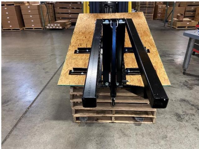
9. Bolt the H-Frame to the extension arms using (2) ½"x 12" hex bolts, (4) nylon washers and (2) ½"
