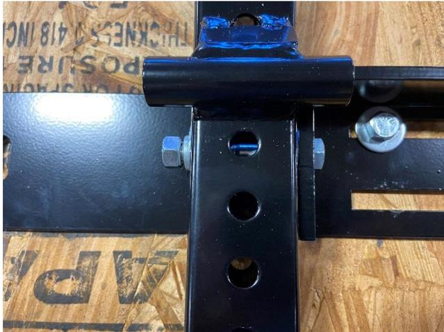
2. Next, using (2) 1/2"x 4 1/2" hex bolts, lockwashers, & hex nuts attach the main support channel to the front pivot tubes welded to the front of the perforated supports as shown in Figure D.
