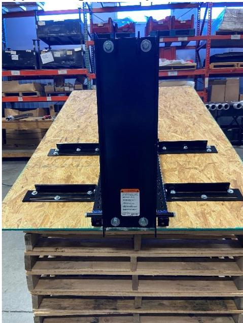
6. Attach the Lower Extension Arms using (1) ½"x 12" hex bolt, (2) nylon flatwashers and (1) ½" locknut. Place one nylon flatwasher between the extension arm and the extension arm support. The nylon washers eliminate paint wear and provide free movement at the pivot points. Remember, the nylon flatwashers go BETWEEN the extension arms and the side of the extension arm support.
