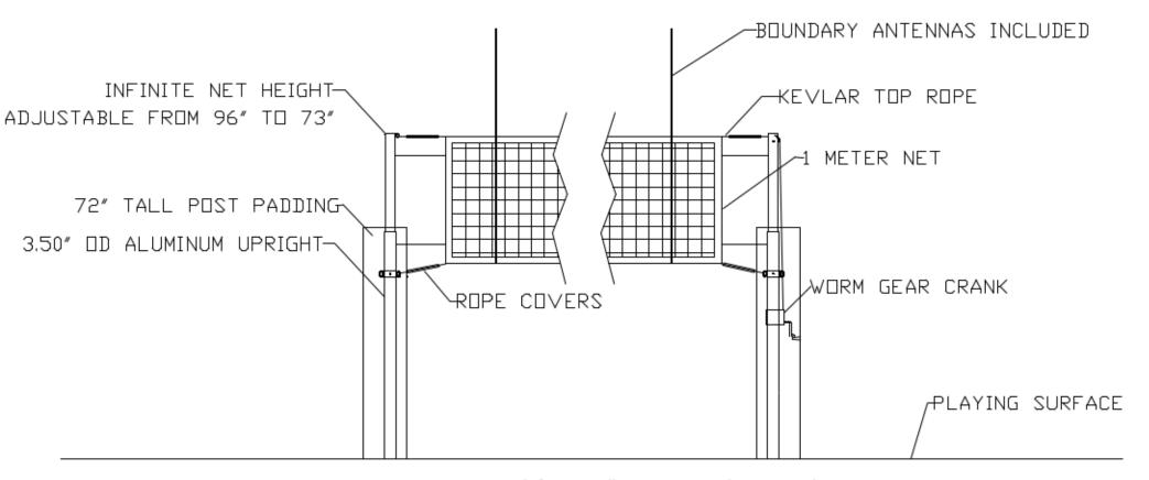
Posts Designed for 3.5" Existing Floor Sockets. First Team will provide socket adapters for other sized floor sockets upon request.
