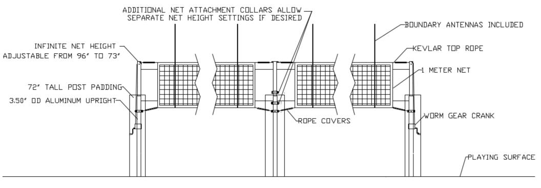
Posts Designed for 3.5" Existing Floor Sockets. First Team will provide socket adapters for other sized floor sockets at no charge upon request.
