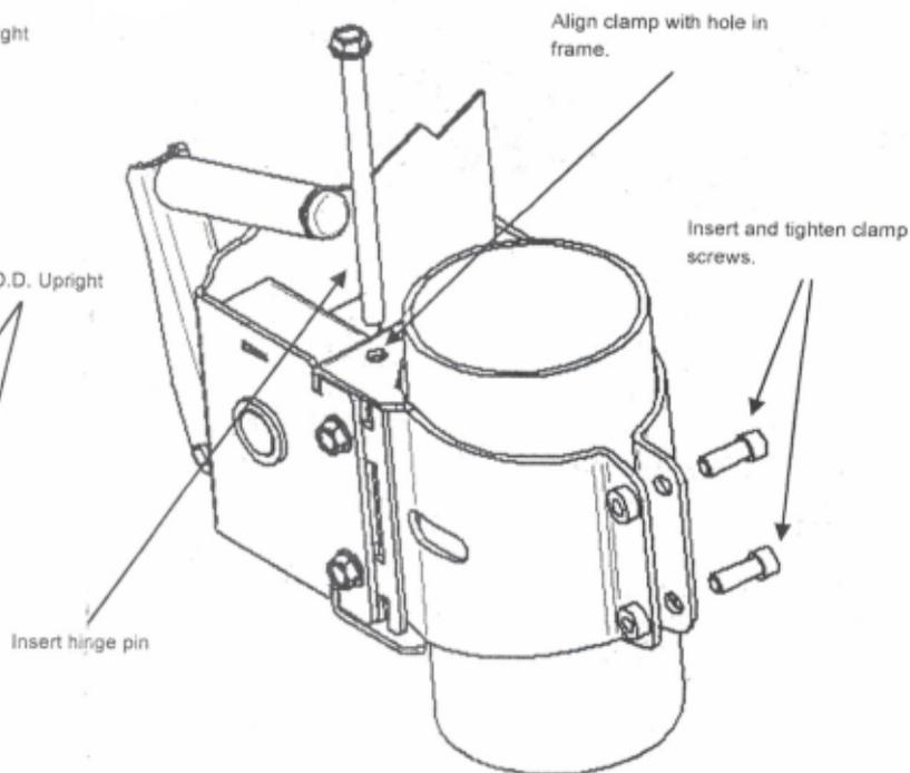
Slip the hinge tabs on the clamps into the winch slots on the winch housing.
