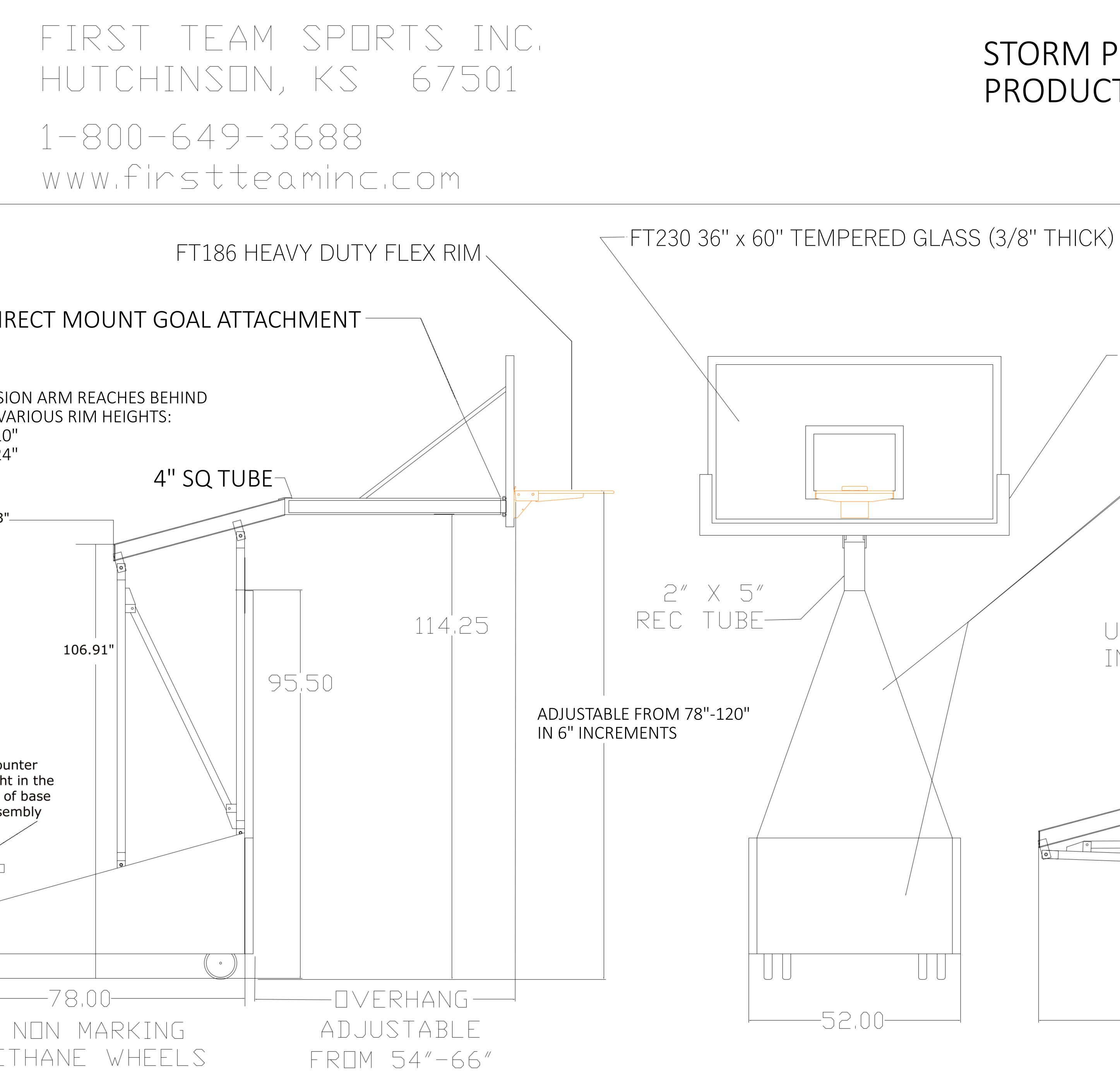
DISTANCE EXTENSION ARM REACHES BEHIND BALLAST BOX AT VARIOUS RIM HEIGHTS: 8' RIM HEIGHT= 10"
