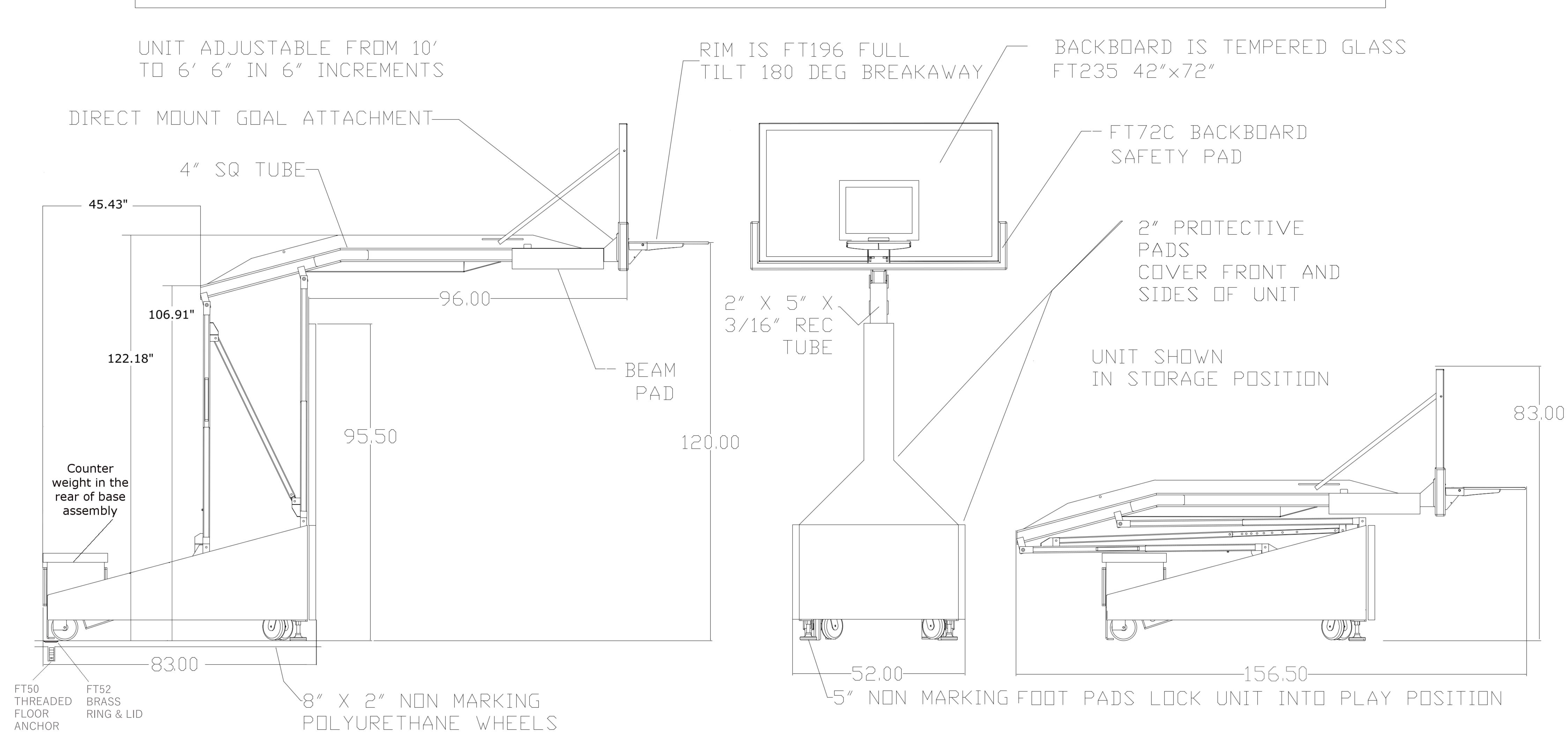
NOTE: ANCHORS FOR A FLOATING FLOOR ARE NOT NEEDED.
