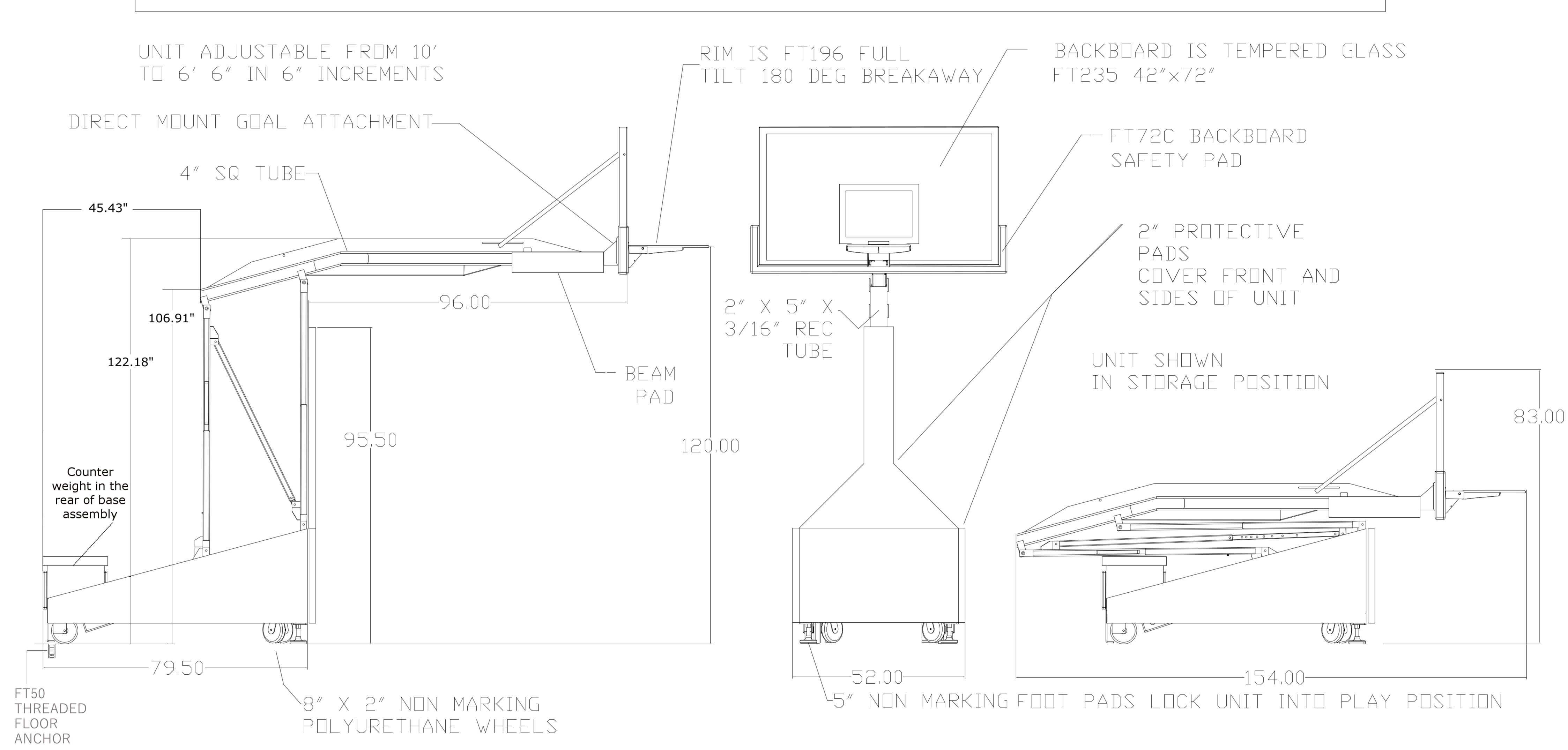
NOTE: ANCHORS FOR A STANDARD FLOOR ARE NOT NEEDED.
