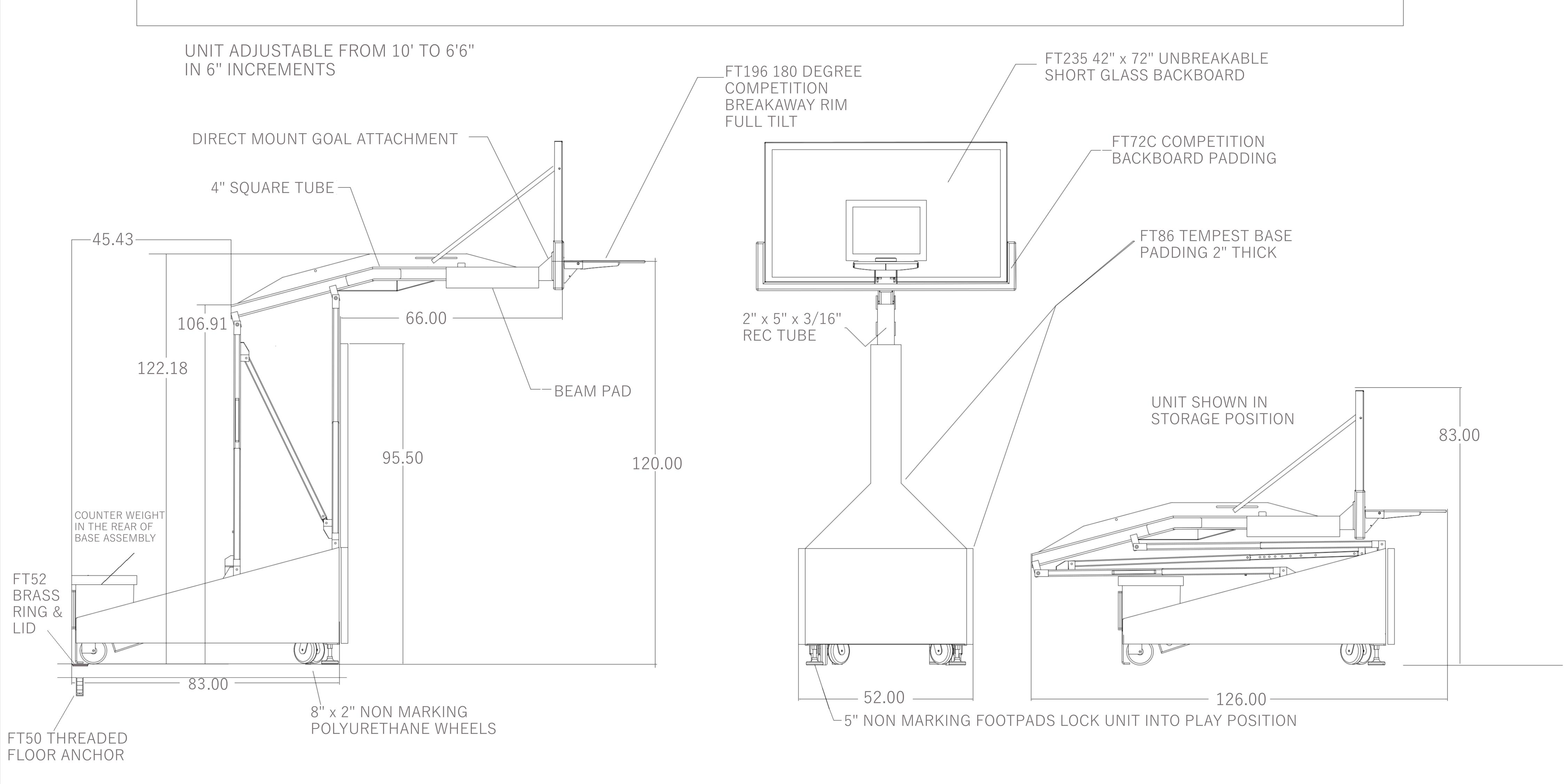
NOTE: ANCHORS FOR FLOATING FLOORS ARE NOT NEEDED. IF YOU DO NOT WANT ANCHORS THEN ORDER THE STANDARD TEMPEST TRIUMPH.
