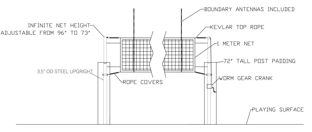
\* POST DESIGNED FOR 3.5" EXISTING FLOOR SOCKETS. FIRST TEAM WILL PROVIDE SOCKET ADAPTERS FOR OTHER SIZED FLOOR SOCKETS AT NO CHARGE UPON REQUEST.
